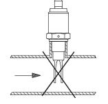
Orientation marking of vibration fork
