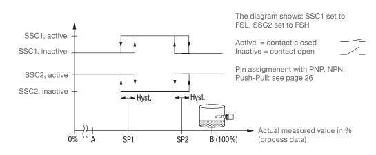
A Used for special application if required (output indicates uncovered)
