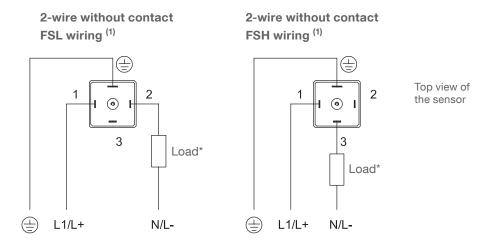
Connect either as FSL wiring or as FSH wiring, depending on required output logic (see below) External fuse in L1/L+: max. 0,5A, fast or slow, HBC, 250V
