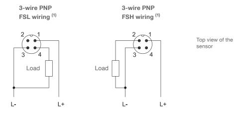
Connect either as FSL wiring or as FSH wiring, depending on required output logic (see below) If required, both outputs (pin 2 and pin 4) can be connected (antivalent). External fuse in L+: max. 0,5A, fast or slow, HBC, 250V
