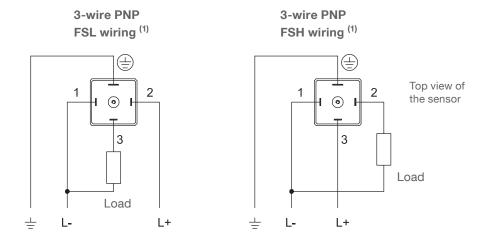
Connect either as FSL wiring or as FSH wiring, depending on required output logic (see below) External fuse in L+: max. 0,5A, fast or slow, HBC, 250V
