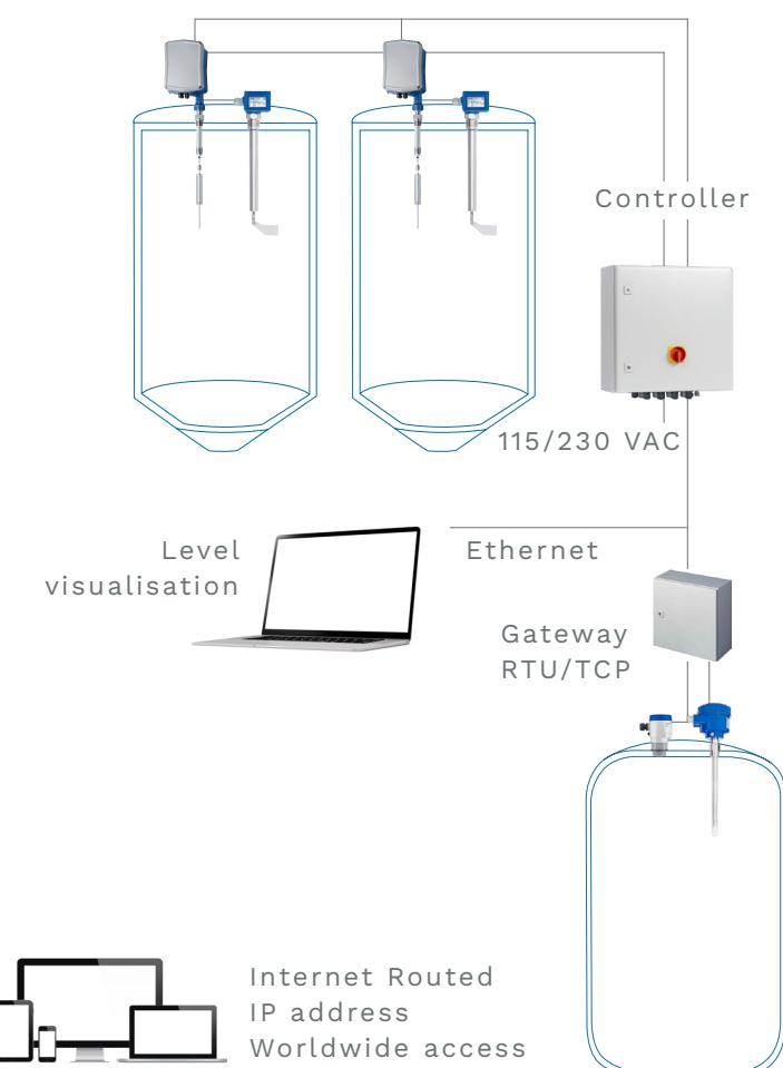
Example of a complete visualisation system for NT 3500 / 4500
